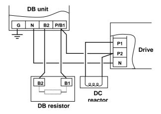
3) Wiring Drive, DB unit, DB resistor and DC reactor
