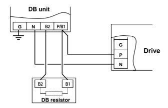
2) Wiring Drive, DB unit and DB resistor for SV030/037/045/055iH-4(Non UL type)
