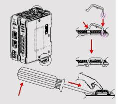
Rail mounting: DIN rail 35mm.
